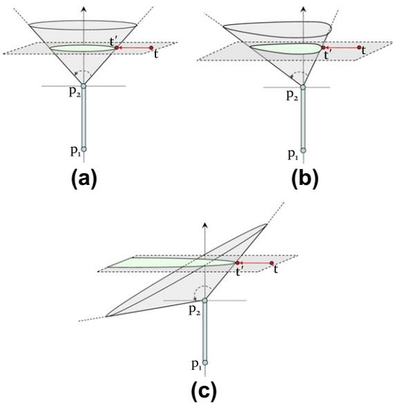
**Fig. 3.** The target is re-positioned within the allowed range of motion which is defined by the conic section. There are 3 types of joint restriction, as described by the angles  $\theta_1, \dots, \theta_4$ : (a) a circle, (b) an ellipsoidal shape and (c) a parabolic shape.
