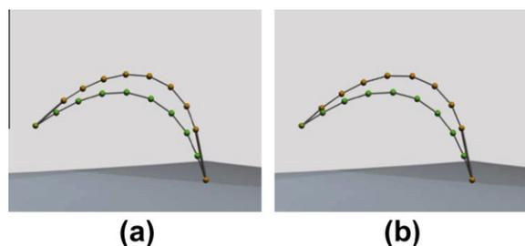
**Fig. 10.** A comparison between the FTL and the FABRIK approaches; the FABRIK posture is shown in green and the FTL posture in orange. (a) The FTL algorithm used fewer averaging iterations to calculate the final pose, thus the resulting posture has more link length variations, (b) the link length variation of the FTL algorithm was reduced over several iterations. Nevertheless, the changes in link size is still significant.
