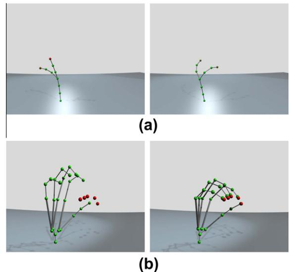
**Fig. 15.** An example of FABRIK implementation with multiple end effectors over time; (a) a kinematic chain with 10 unconstrained joints, 2 end effectors and 2 targets, (b) A hand motion example using FABRIK; this is a fully unconstrained hand example, allowing 3 DoFs on each joint.
