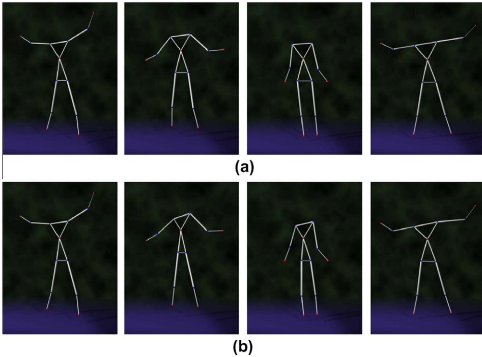
**Fig. 16.** A low rate body tracking example. The joints in red are the known positions of the end effectors and those in blue are the estimated joint positions. (a) shows the true body poses and (b) the estimated poses using FABRIK.
