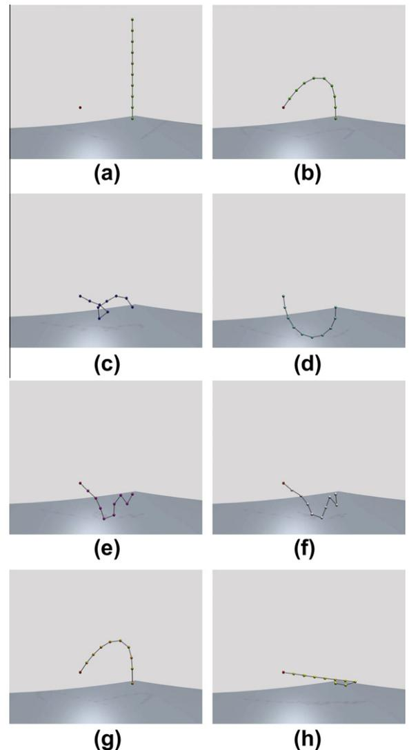
**Fig. 9.** Experimental solutions using some of the most popular IK methods. The kinematic chains consisted of 10 unconstrained joints, allowing 3 DoFs on each joint. (a) Initial position, (b) FABRIK, (c) CCD, (d) J. Transpose, (e) J. DLS, (f) J. SVD-DLS, (g) FTL, (h) Triangulation. Note that the link lengths of the resulting FTL posture are not equal to their initial size.
