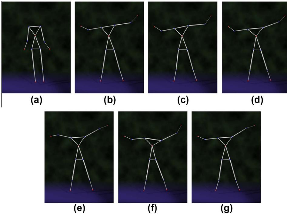
**Fig. 17.** Body reconstruction using different IK methodologies. The joints in red are the known positions of the end effectors and those in blue are the estimated joint positions. (a) shows the initial position and (b) the true final position. (c) shows the FABRIK solution, (d) the CCD solution, (e) the J. Transpose solution, (f) the J. DLS solution, (g) the J. SVD-DLS solution
