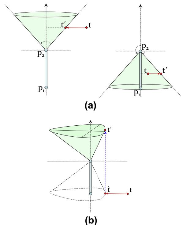
**Fig. 6.** Solution for special joint restriction cases: (a) the original case and when the allowed range of motion is greater than 180 degrees, (b) when the target is located on a different hemisphere than the irregular cone.
