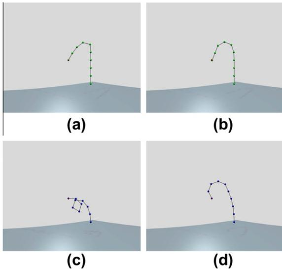
**Fig. 18.** An example of FABRIK and CCD implementations with and without incorporating constraints. (a) presents the FABRIK unconstrained solution and (b) the FABRIK constrained solution. (c) presents the CCD unconstrained solution, and (d) is the CCD constrained solution.
