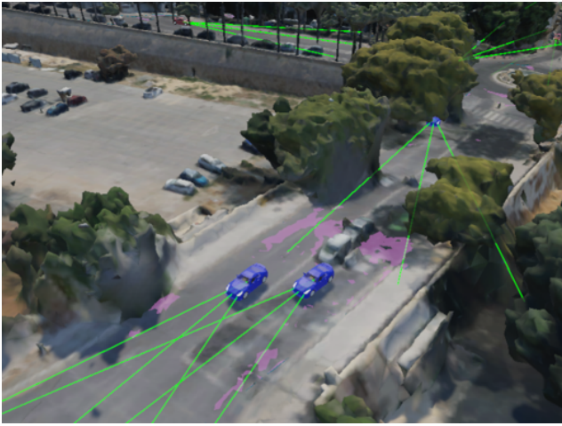
Figure 4: A snapshot of vehicle simulation within a 3D model of Nicosia. A ray-cast system enables vehicle collision avoidance by detecting frontal obstacles and adjusting throttle accordingly.
