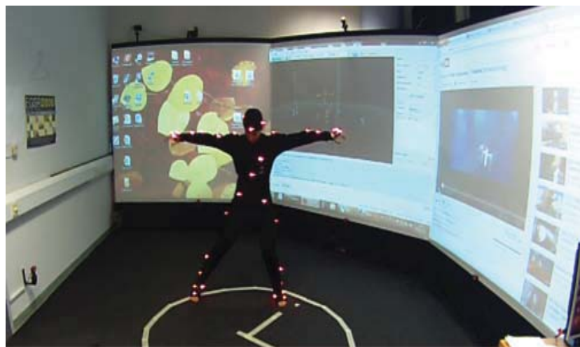
Figure 3.1 A dancer wearing a motion capture suit at VRL, where its movements are captured using the PhaseSpace Impulse X2 motion capture system.
